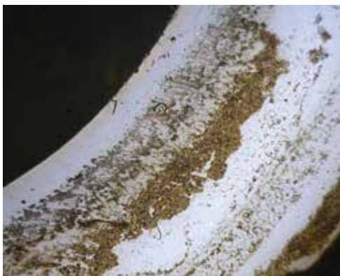
Seat Deformation & Heavy Debris Build-up Caused Seat Leakage
